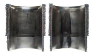
The image on the right shows damage from wear, and the image on the left show the protection provided by Performance Plus.
