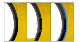
Performance Plus<sup>®</sup> Synthetic Blend High Mileage Passenger Car Motor Oils are blended with a special additive package designed for older vehicles or those with high miles ( $\geq$  70,000 miles). These additives cause a chemical reaction with the elastomeric seals and gaskets to cause a slight sw ell to improve protection and aid in the sealing of leaks all the w hile continuing to provide sludge and deposit control.
